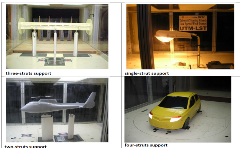
Figure 7: Assembly of model support system to accommodate various types of testing.
