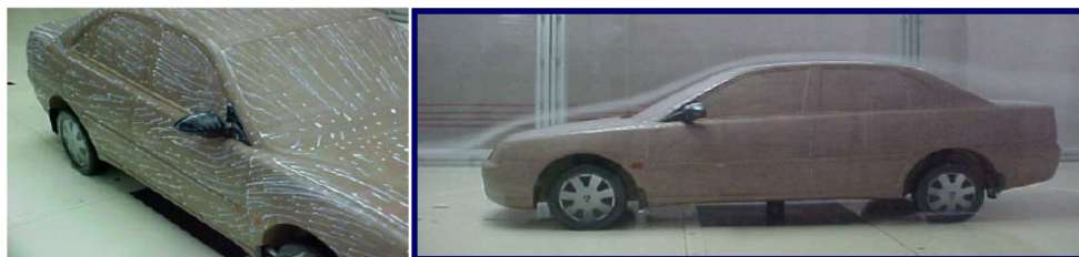
Figure 9: Flow visualization using smoke and oil.
