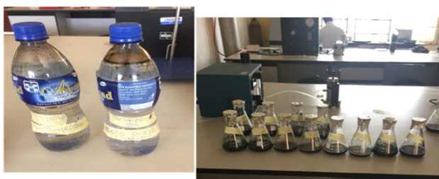
Figure 1.1: Sample of produced water and filtrates from the adsorption column.
