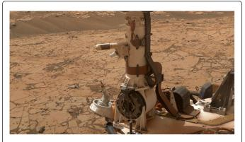
Figure 1: Image of REMS's boom 2 on Curiosity's Mast.
