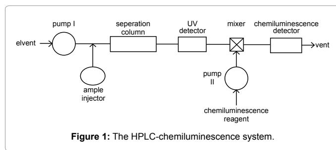
Figure 1: The HPLC-chemiluminescence system.
