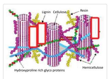
Figure 1: Wood microscopic structure showing the lignin position within lingocellulosic matrix [24].
