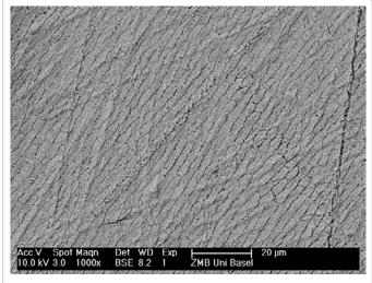
Figure 1: Typical surface after conventional etching with 37% phosphoric acid for 30s.
