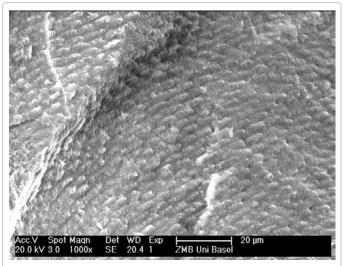
Figure 2: Surface structure after CO2 laser. A microretentive relief can be seen on the enamel.
