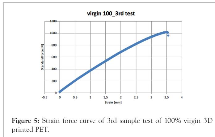
Figure 5: Strain force curve of 3rd sample test of 100% virgin 3D printed PET.
