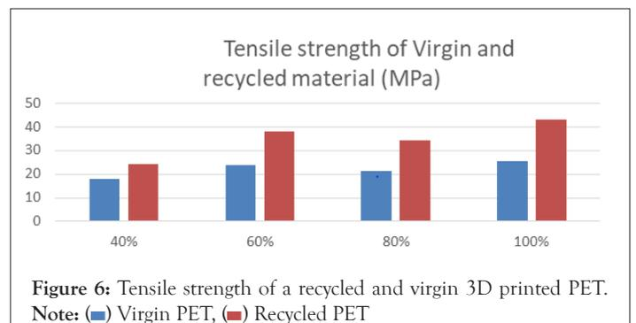
Figure 6: Tensile strength of a recycled and virgin 3D printed PET. Note: (■) Virgin PET, (■) Recycled PET
