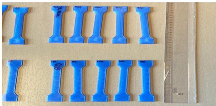
Figure 2: Testing materials standard for the specimens.
