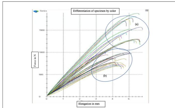
Figure 4: Tensile Elongation of a recycled (a) and virgin (b) 3D printed PET.
