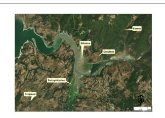
Figure 8: Increased of cropland areas caused the eutrophication and siltation in Aslantaş Dam.
