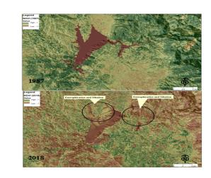
Figure 9: Siltation and eutrophication events intensive North and east side of Aslantaş Dam (1987 and 2018).
