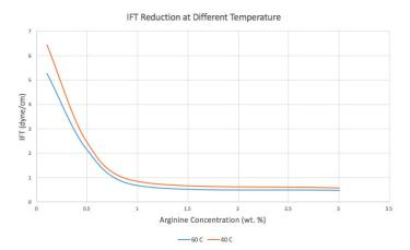
Figure 3: IFT at different temperature.
