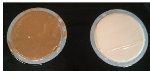
Figure 6: Mud cake of Base mud (Left) and Nano-WBM (Right).
