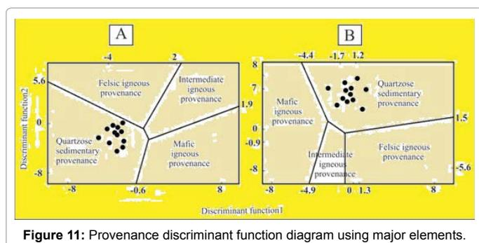
**Figure 11:** Provenance discriminant function diagram using major elements.
