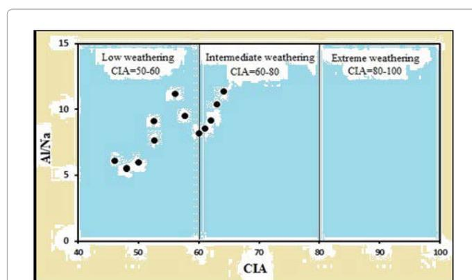
**Figure 14:** Scatter plot of Al/Na ratios versus Chemical Index of Alteration (CIA) for the studied samples. Fields are from Servaraj and Arthur (2006).
