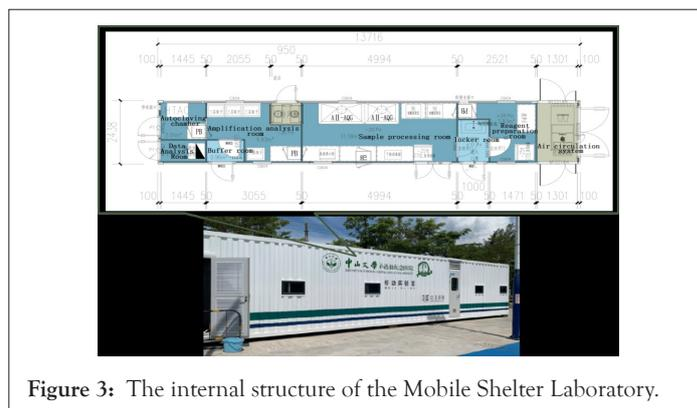
Figure 3: The internal structure of the Mobile Shelter Laboratory.
