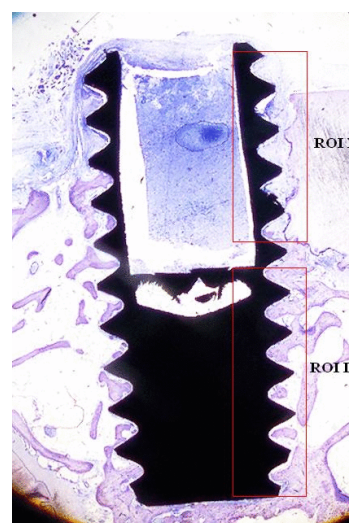
Figure 1. Shows ROI I & ROI II. ROI I corresponds to the coronal threads embedded in dentin and ROI II corresponds to the apical threads embedded in host bone.
