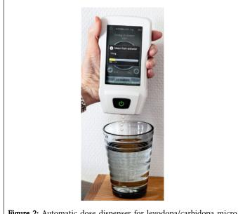
**Figure 2:** Automatic dose dispenser for levodopa/carbidopa micro tablets [28].
