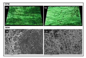
**Confocal Miscrocopy (CFM).** X20 Three-dimensional reconstruction of a  $2 \times 2$  mm area of root surface. Note that the closer cool and warm colors turn green and shadows tend to disappear as the surfaces becomes smoother.
