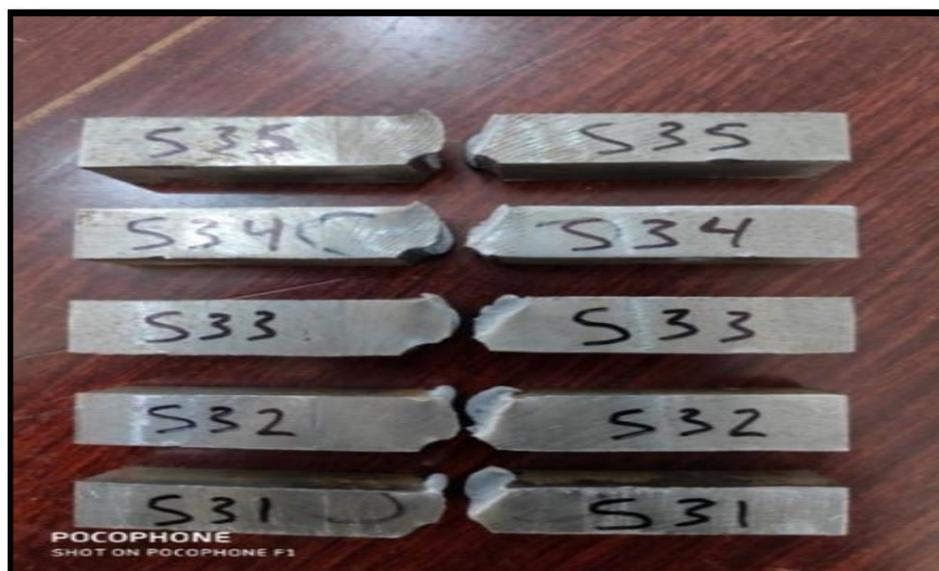
Figure 2: Impact specimens after the test.
