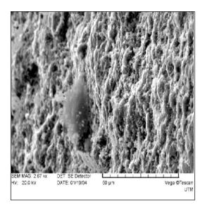
Figure 2. Surface processed by anode oxidation
