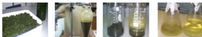
(Algae) (Oil extraction) Extrated oil Biodiesel (I: single, II: mixture) Fig. 1. Shows the oil extraction and biodiesel yield from Spirogyra sp. algae
