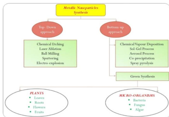
Figure 1: Metallic Nanoparticles synthesis.
