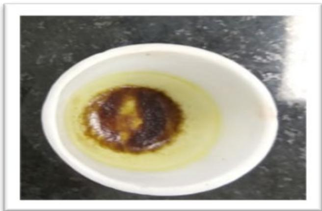
Figure 4: Dried sample in crucible.
