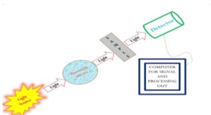
Figure 6: Working of UV-Vis Spectrophotometer.
