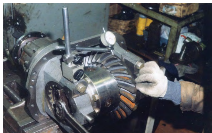
Figure 3: Adjustment of interlocking parameters and preload of differential bearings in the gearbox of the drive axle of automobile.
