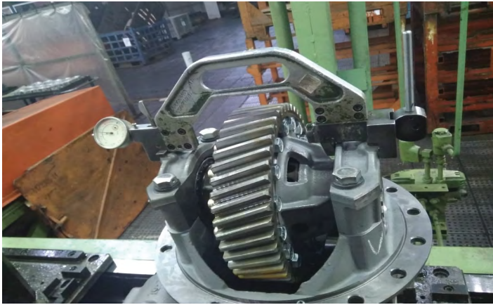
Figure 8: Technical equipment for the adjustment of the preload of differential bearings in the drive axle gearbox in real production.
