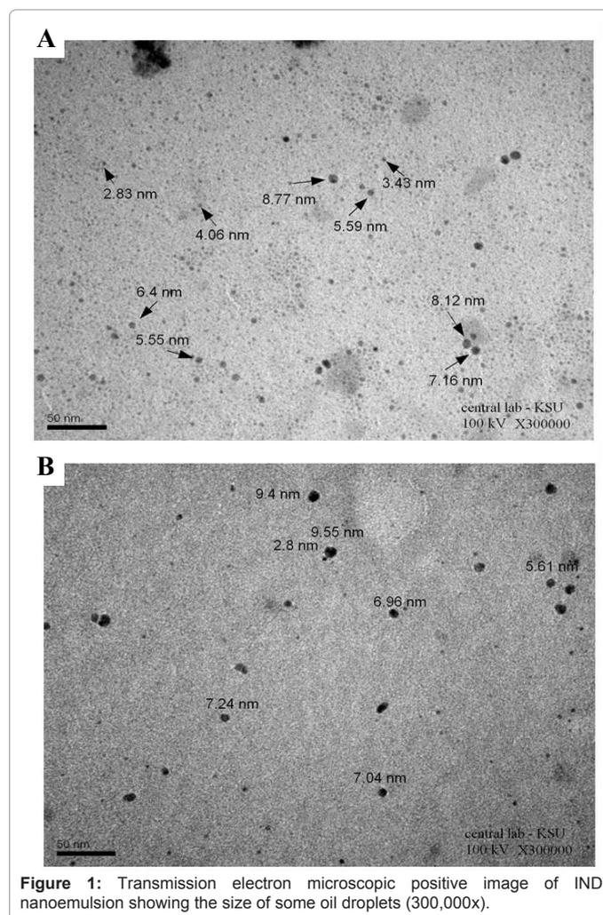
Figure 1: Transmission electron microscopic positive image of IND nanoemulsion showing the size of some oil droplets (300,000x).
