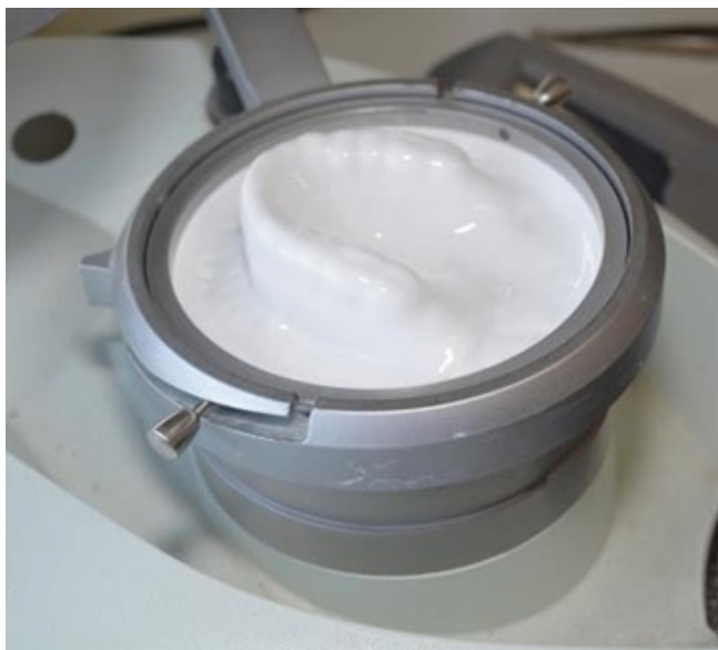
Figure 5: Heating and suction of the EVA sheet by the vacuum forming unit.
