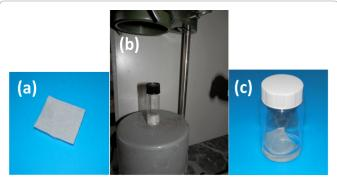
**Figure 1:** Fabric phase sorptive extraction: (a) a fabric phase sorptive extraction (FPSE) device; (b) extraction using FPSE device; (c) solvent mediated back-extraction.
