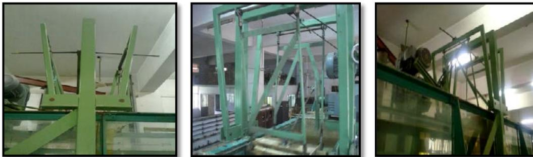
Figure 3: Electric motor type wave generator used in laboratory experiment.
