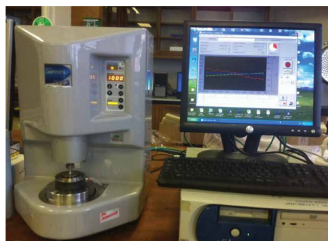
Figure 1: A Bohlin Gemini II Rheometer was used to determine pour point, viscosity and WAT of the crude oil before and after adding the inhibitors.
