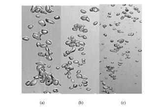
**Figure 6:** Example of photograph of bubbles at  $u_z$ =0.13 cm/s for SDS/water system; (a)  $C_z$ =0.02% vol; (b)  $C_z$ =0.05% vol; (c)  $C_z$ =0.1% vol.
