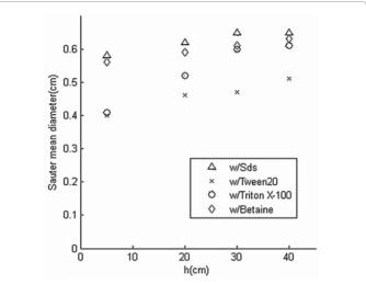
**Figure 9:** Sauter mean bubble diameter as a function of distance from gas sparger.
