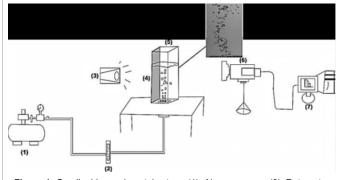
**Figure 1:** Gas-liquid experimental set-up. (1): Air compressor (2): Rotameter (3): Halogen lamp (4): Plexiglas plate (5): Bubble column (6): Camera (7): Image processing.
