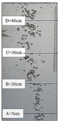
**Figure 2:** Photograph taken from different location of column in Tween20/ water system at  $C_s$ =0.05% vol and  $u_a$ =0.13 cm/s Location A , B, C and D.
