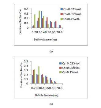
Figure 5: Influence of SDS concentration upon bubble diameter at  $u_{z}$ =0.13cm/s; (a) Location A. (b) Location D.
