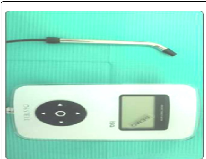
Figure 7. Osstell ISQ device.
