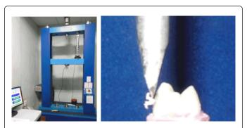
**Figure 3:** (a) Universal testing machine, (b) Premolar with bracket bonded and the chisel tip acting in the upper part of the bracket base during shear bond strength test
