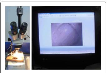
Figure 4: Stereoscopic magnifying glass along with its magnified image (10X)
