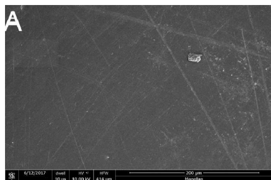
Figure 4: Composite surface after 24 h exposure to Oral Essentials® Whitening Strips. A: X500; B: X3000. SEM.
