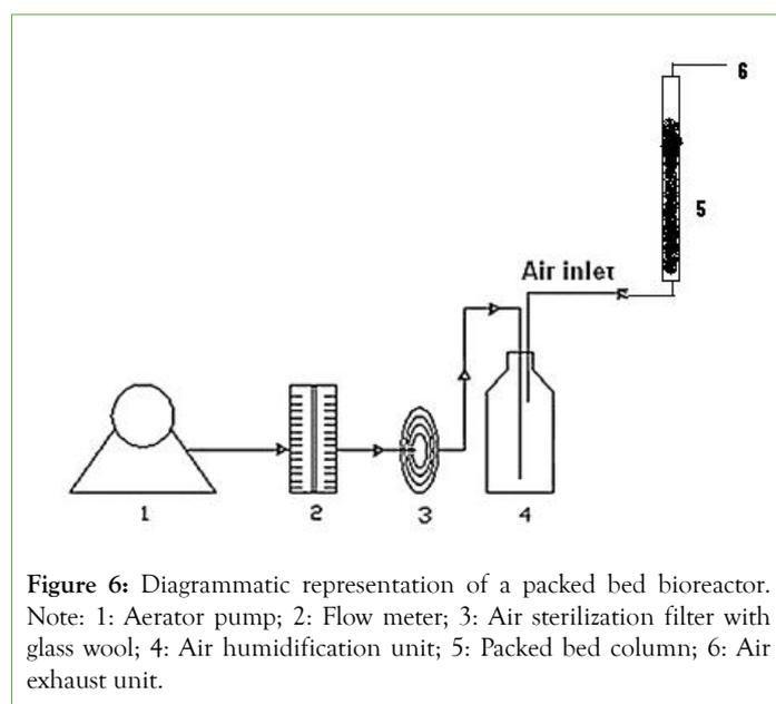
**Figure 6:** Diagrammatic representation of a packed bed bioreactor. Note: 1: Aerator pump; 2: Flow meter; 3: Air sterilization filter with glass wool; 4: Air humidification unit; 5: Packed bed column; 6: Air exhaust unit.**Table 5:** Effect of aeration on packed bed bioreactor for production of  $\alpha$ -galactosidase by *B. megaterium* VHM1.
