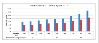
**Figure 3**: Effect of fermentation temperature and agitation speed on methane yield.
