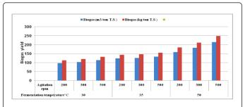
**Figure 2**: Effect of fermentation temperature and agitation speed on cumulative biogas production.
