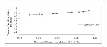
**Figure 9**: The comparison between the predicted and the measured degradation efficiency (De) during biogas production at 3 day.
