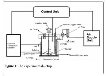
The experiment was devoted to study the effect of fermentation temperature (FT) and agitation speed(AS) on cumulative biogas production from dairy manure anaerobic fermentation as affected by temperature with (30, 35 and 50°C) and agitation rotation speed (200, 300, and 500 rpm). A total of 27 runs including 3 replicates were conducted.
