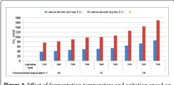
**Figure 4**: Effect of fermentation temperature and agitation speed on carbon dioxide.
