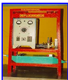
Figure 2: The electrochemical removal of fluoride from drinking water based on electrocoagulation process is already commercialized. The process involves the generation of aluminum hydroxide by the anodic dissolution of aluminum, which adsorbs the fluoride and settles.
