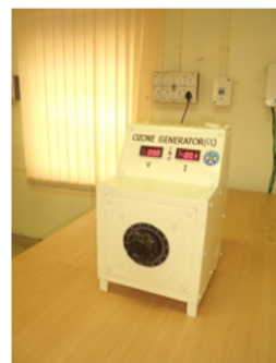
Figure 4: Electrochemical ozone generator based on PEM technology has been tested in the laboratory scale and a portable ozone generator.
