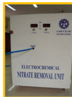
Figure 5: The electrochemical removal of nitrate from drinking water based on reduction cum oxidation process is successfully developed.
