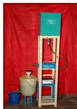
Figure 3: The electrochemical removal of arsenic from drinking water based on electro coagulation process.
