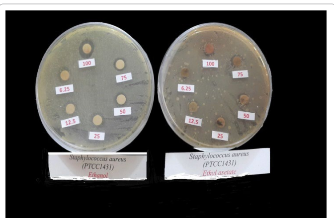
Figure 1: Disc diffusion assay showing inhibition zone induced by several concentrations of ethanolic/ethyl acetate extracts of E. helioscopia against S. aureus .
