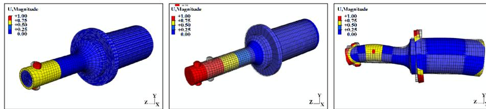
Figure 1: Numerical shapes of the torsional (13.2 kHz), operating (20.8 kHz) and bending (22.6 kHz) mode.
