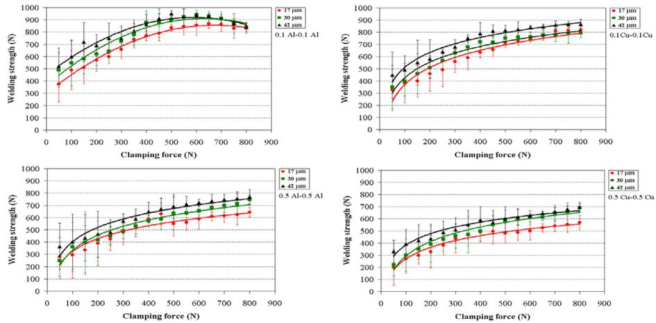
Figure 4: Variation of weld strength vs. clamping force for joining similar materials.
