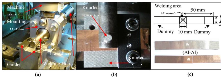
Figure 3: Experimental set up of welding tools, knurled surfaces, specimen layout and welded coupons.
