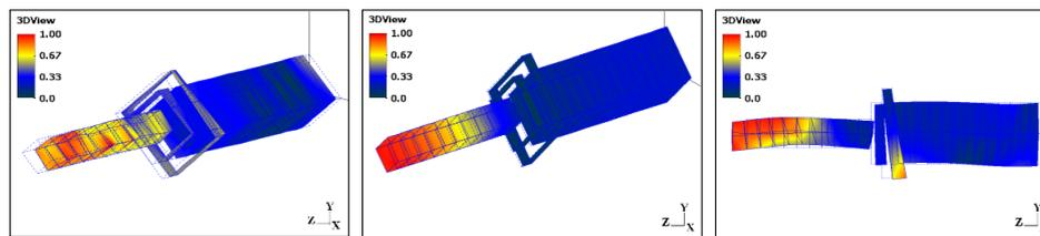
Figure 2: EMA shapes of the torsional (13.7 kHz), operating (20.8 kHz) and bending (23.5 kHz) mode.
