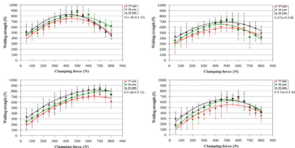
Figure 5: Variation of weld strength vs. clamping force for joining dissimilar materials.
