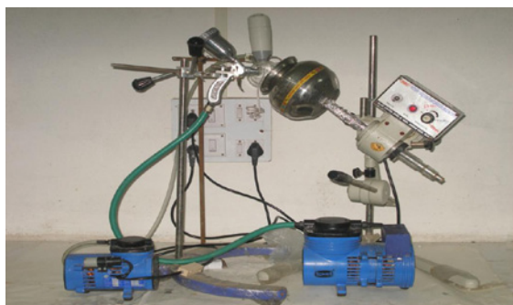
Figure 2: Spray coating pan fabricated in the laboratory.
