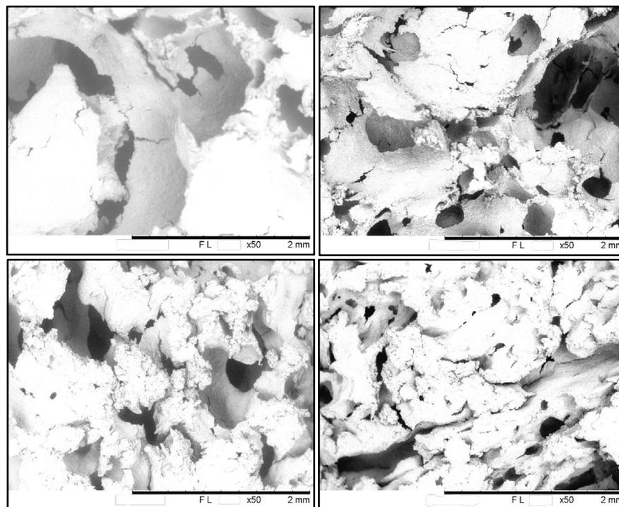
**Figure 7:** Scanning electron micrographs of crumb of three SBY-fortified composite bread (cassava-wheat) and control (without SBY) at the magnification  $\times 50$  (a) Control (without SBY) (b) 5% SBY, (c) 10% SBY (d) 15% SBY.
