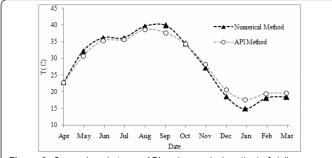
Figure 6: Comparison between API and numerical method of daily average tank temperature.
