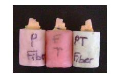
Figure 3: Fractured composite cores, leaving almost half the cores bonded to the fiber dowels. Fracture extended along the core dowel interface in all samples.
