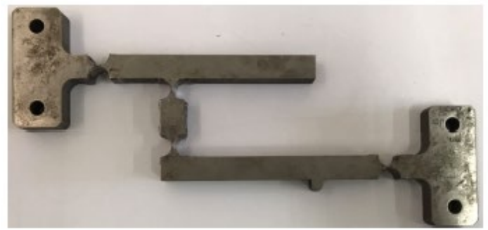
Figure 10: Flexure hinges before added with damping material.
