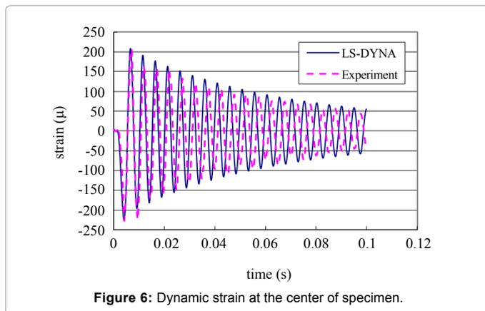
Figure 6: Dynamic strain at the center of specimen.
