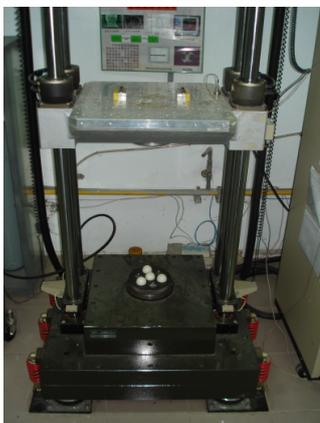
Figure 1: Experimental setup of drop test.
