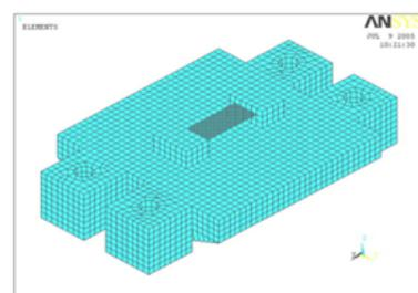
Figure 3: Finite element mesh of the drop table and test specimen.
