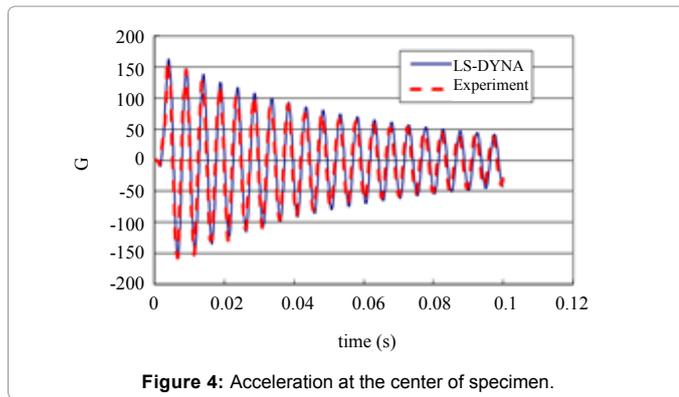
Figure 4: Acceleration at the center of specimen.
