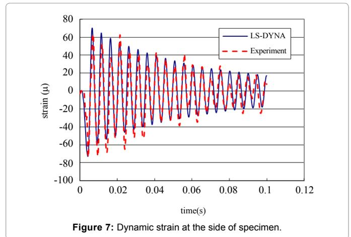
Figure 7: Dynamic strain at the side of specimen.
