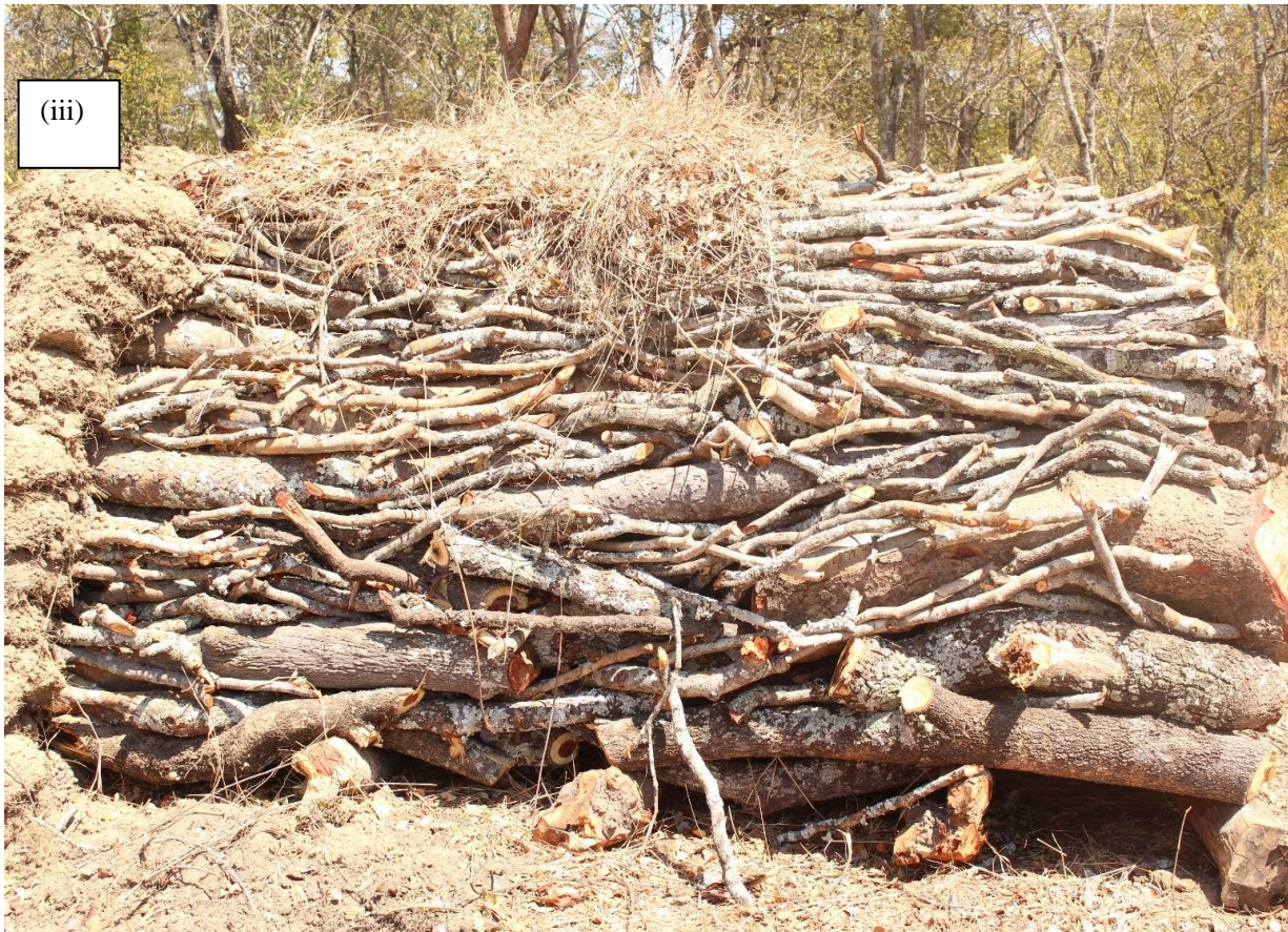
Figure 6: Building a charcoal kiln, (i) felled tree cut into desirable log lengths and (ii and iii) logs piled to build an earth kiln before pyrolysis
