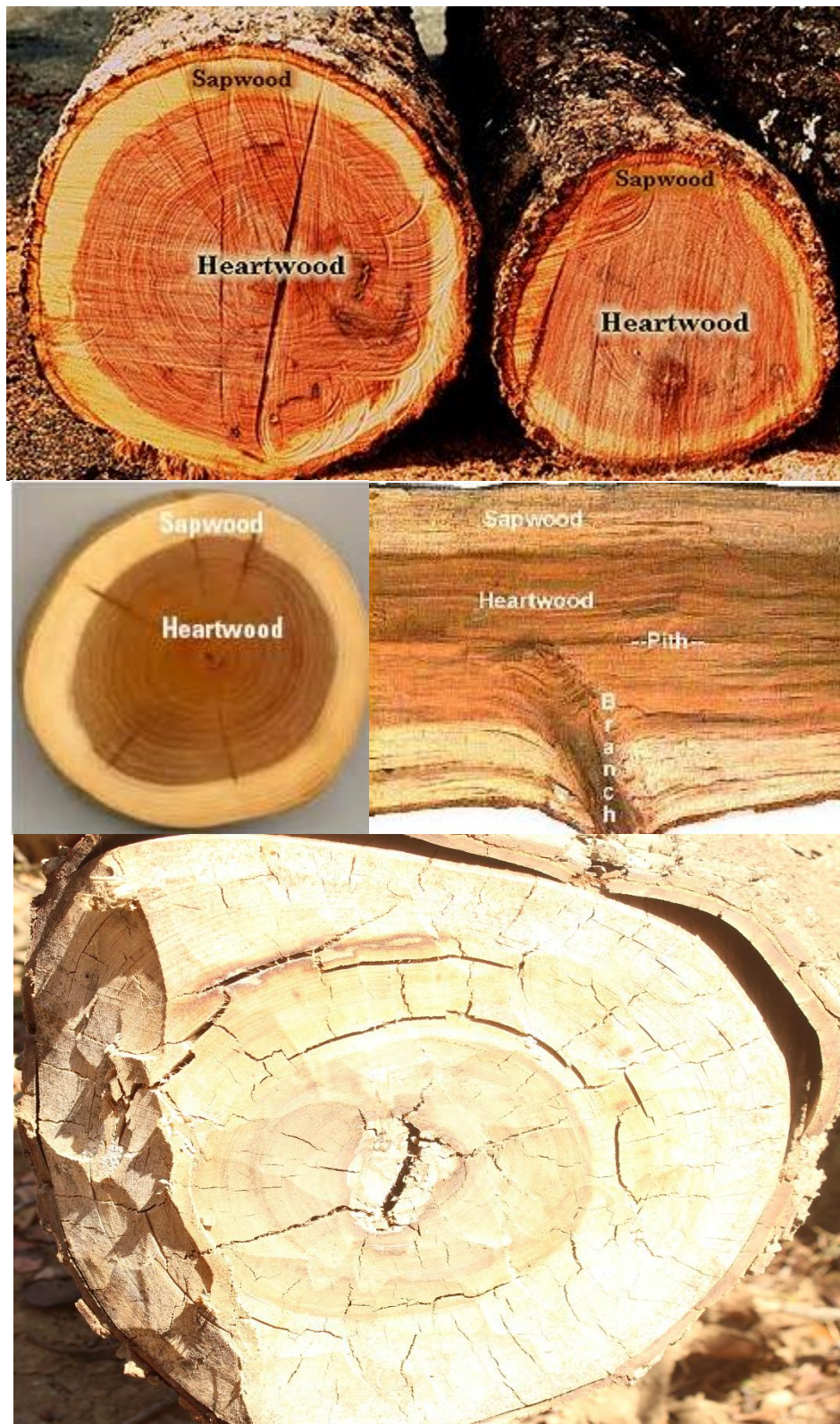
Figure 5 Stem transverse section showing sapwood (lighter area) and heart wood (darker area) a) as adopted from Microsoft Encarta, 2009; http://www.google.com downloaded on 8 th February 201) and b) Brachystegia spiciformis cut for charcoal production in the study area.
