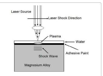
Figure 2: Schematic of laser shock processing on magnesium alloy [11].
