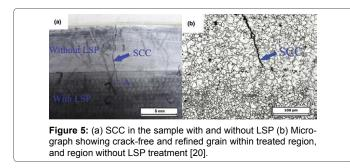
so that compressive residual stress is formed on the surface layer of the material, which can then be used to balance tensile stresses when it is in working condition, thereby preventing the generation of stress corrosion cracking, and preventing the growth of stress corrosion cracks, as shown in Figure 5 [20].
