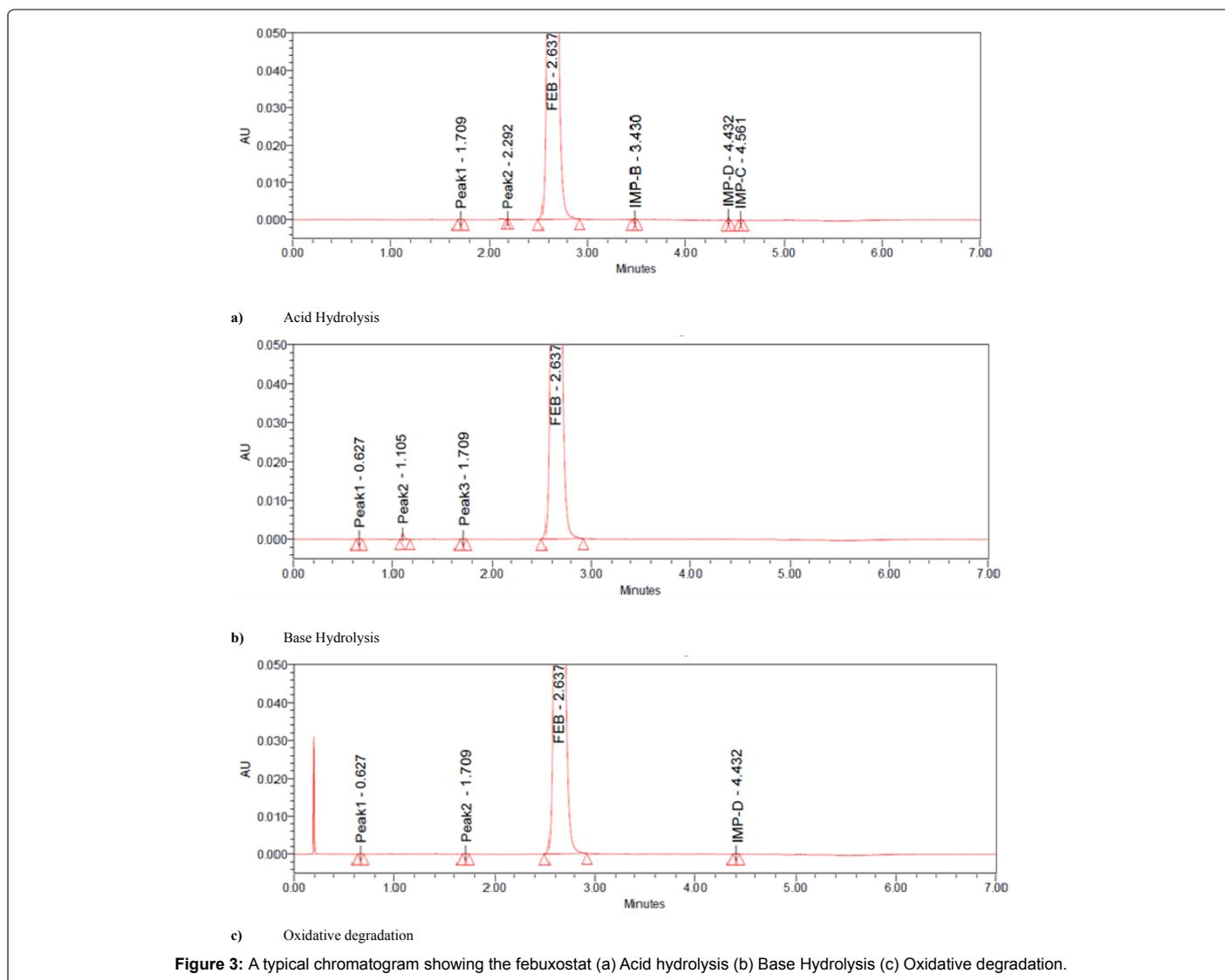
Figure 3: A typical chromatogram showing the febuxostat (a) Acid hydrolysis (b) Base Hydrolysis (c) Oxidative degradation.
