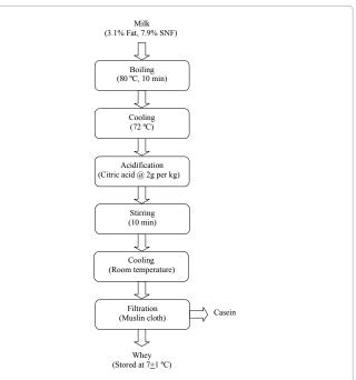
Figure 2: Process flow diagram for the milk whey preparation.
