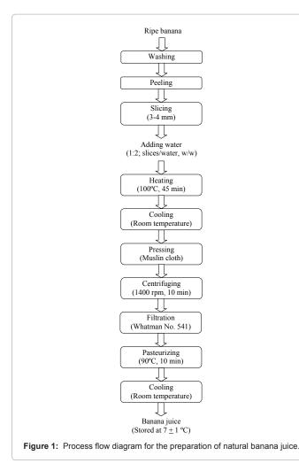
slices of 3-4 mm. The banana slices along with RO purified water in the ratio of 1:2 (banana slice : water, w/w) were heated at 100°C for 45 minutes followed by the cooling, pressing, centrifuging (at 1400 rpm for 10 min), filtration, pasteurization (at 90°C for 10 min) and again cooling at room temperature. The prepared banana juice was stored at  $7 \pm 1$ °C temperature in the refrigerator for further use in the RTS beverage preparation.
