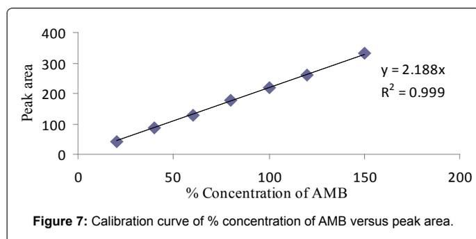
Figure 7: Calibration curve of % concentration of AMB versus peak area.
