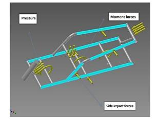
Figure 4: Frame with Pressure, Moment Forces and Side Impact Forces Points.
