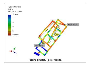
has been generated. The value of histogram varied from max. to min. with their color contrast (Table 7). According to the values factor of safety obtained is 3 and max as shown in Figure 8.
