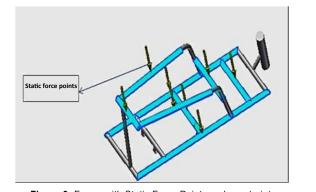
Figure 3: Frame with Static Force Points and constraint.
