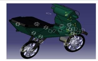
Figure 1: CATIA V5 design image of the two wheeler EV IGNITIA V1.0, side view [4].
