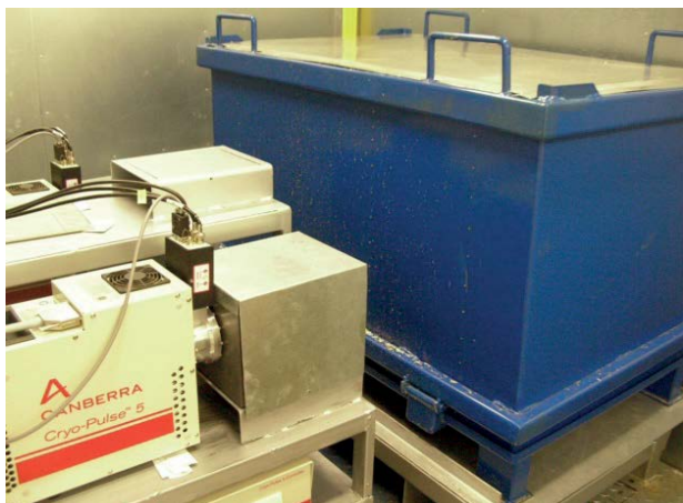
Figure 1: Detectors and shielding arrangement on rack during container measurement .
