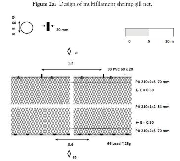
Figure 2b: Design of multifilament shrimp gill net.
