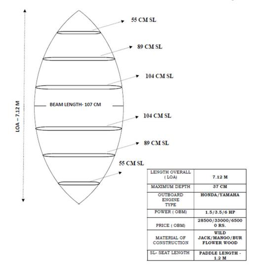
Figure 4: Technical specification of traditional wooden canoe.
