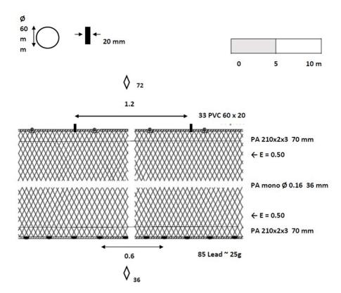
Figure 3b: Design of monofilament shrimp gill net.
