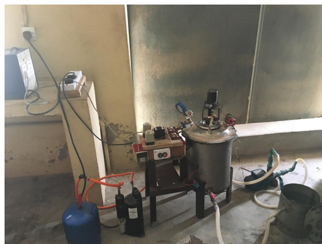
Figure 7: Image of the fabricated jacketed batch bio-digester system showing all components.
